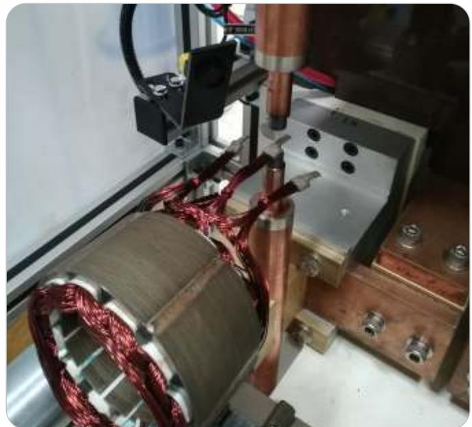
Resistance welding is used to burn enamel and crimp multi-strand wires to lugs. It differs from other types of resistance welding because it uses a conductive metal sleeve to pass the current, generate the heat and hold the wires together. Wires & lugs of different combinations can be used.
